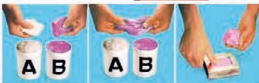
Smooth consistency mouldable rubber: Fast reacting, cures in only 3 minutes. The result is more rigid and less elastic than GSP-400, yet maintains a high fidelity to original. Suitable for quickly producing small moulds or for directly making casts of parts of the body, hands or face. The rubber is absolutely nontoxic and hypoallergenic, therefore does not cause irritation to the skin.
