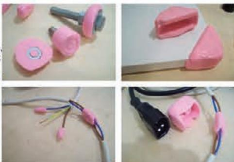
Two component, insulating paste rubber, moldable, flame retardant; Once mixed the 2 components in a 1:1 ratio (for not mote than 2 min.) and obtained a uniform compound, it rapidly cures at room temperature in less than 5 minutes.
